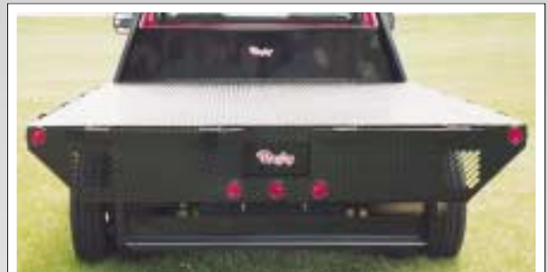
Clearance lights are recessed flush with rub rail
